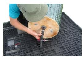
9. Connect the tubing to the pump and clamp.
